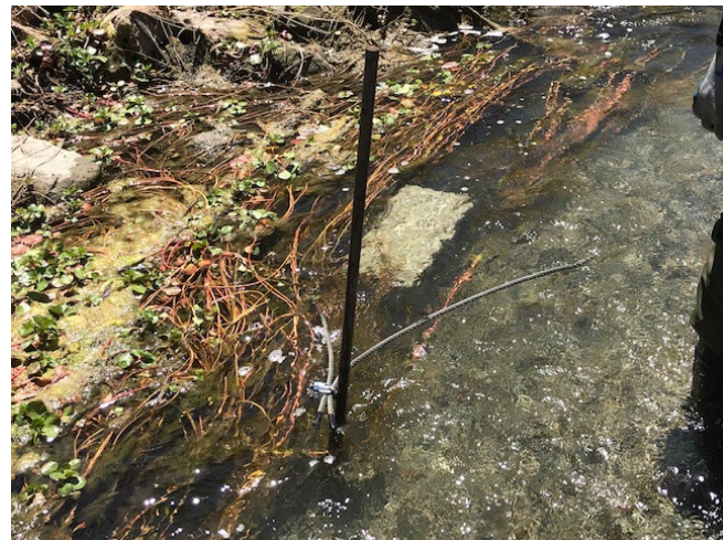
Figure 5-16: A Hobo MX2201 temperature sensor secured using 3/8 th -inch steel cable to steel stake, driven into channel bed.
