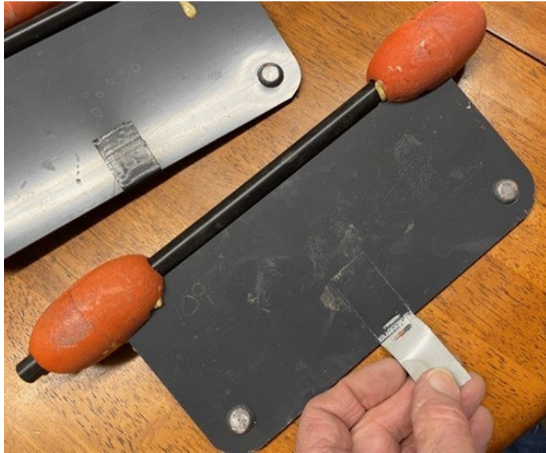
Figure 4-4: Customized float apparatus from West Fork Environmental to hold test PIT tags.
