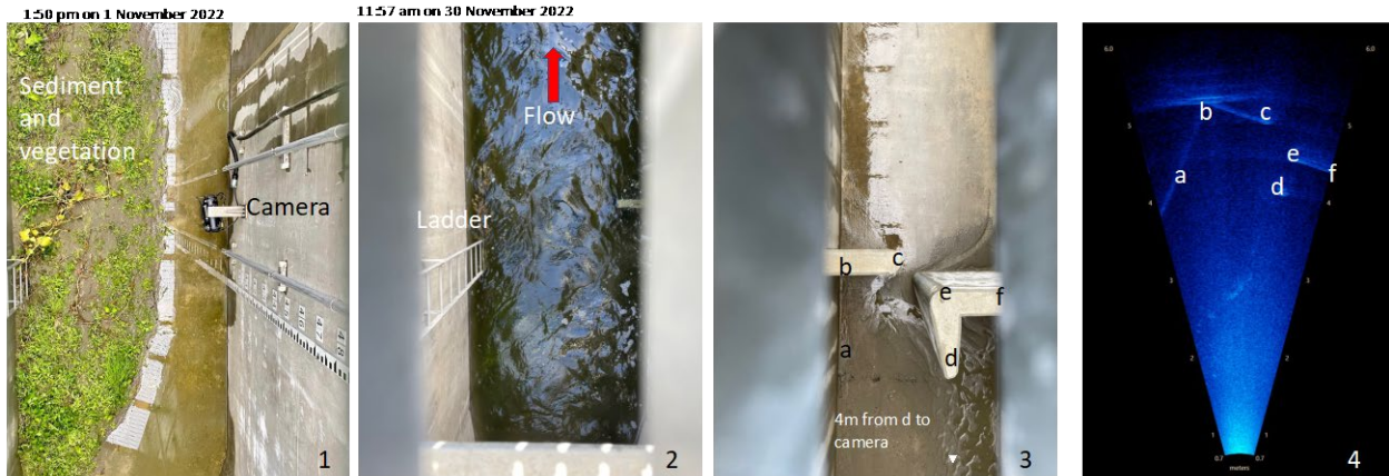
Figure 4-13: Image 1 demonstrates ARIS bay dry. Note sediment and moisture allow terrestrial vegetation colonization (taken 1 November 2022). SONAR camera is facing downstream. Camera mount is ~ 61 cm above concrete floor. Image 2 demonstrates the ARIS bay with passage flow; Camera and mount submerged. Water depth is ~65 cm. Image 3 shows demonstrates downstream opening to ARIS bay. Note corresponding letters in SONAR image (Image 4).
