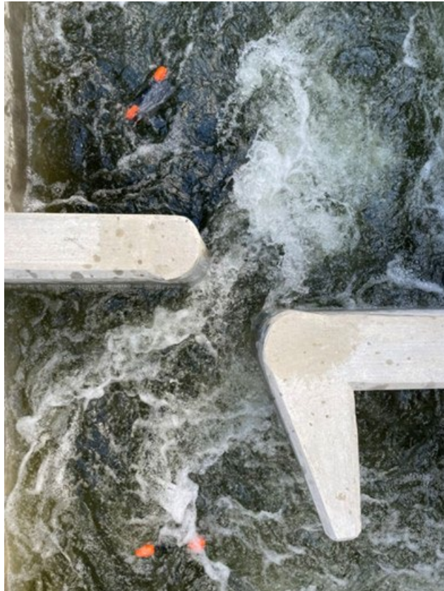
Figure 4-5: Example of two tags floating through a ladder bay. Flow is moving from bottom of photo up. Note this bay does not have an antenna and the image is for illustration purposes only.
