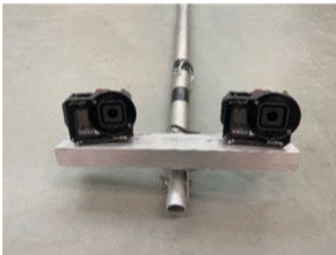
Figure 5-2: GoPro stereo-camera system mount on adjustable ~15ft aluminum pole.
