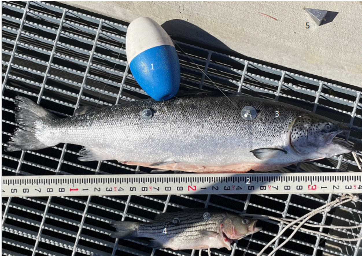
Figure 4-3: Testing of the ARIS sonar camera using market fish. (1) Float used to keep fish oriented and off channel bottom; (2) Stadia rod used to take water depths and hold weight and can in place; (3) 83.21 cm Atlantic Salmon (4) 38.10 cm Striped Bass; (5) 5.08 cm 8-ounce weight. The reference aluminum can is not shown.
