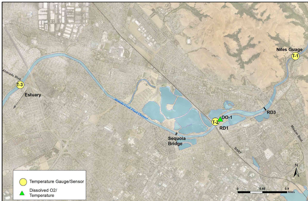
Figure 5-17: Map of temperature and dissolved oxygen sensors. (T-1) is the temperature sensor at USGS Nilas Gauge (USGS 11179000); (T-2) is a set of sensors within the RD1 Fish Ladder, one near the entrance gate at the downstream end of the upper fish ladder, and the other is near the exit gates by the trash rack on the upstream end of the fish ladder; (T-3) is in the flood channel at Alvarado Blvd. bridge. The green triangle is the location of a dissolved oxygen and temperature sensor, located in the RD1 forebay, near the trash rack, approximately mid-water column.
